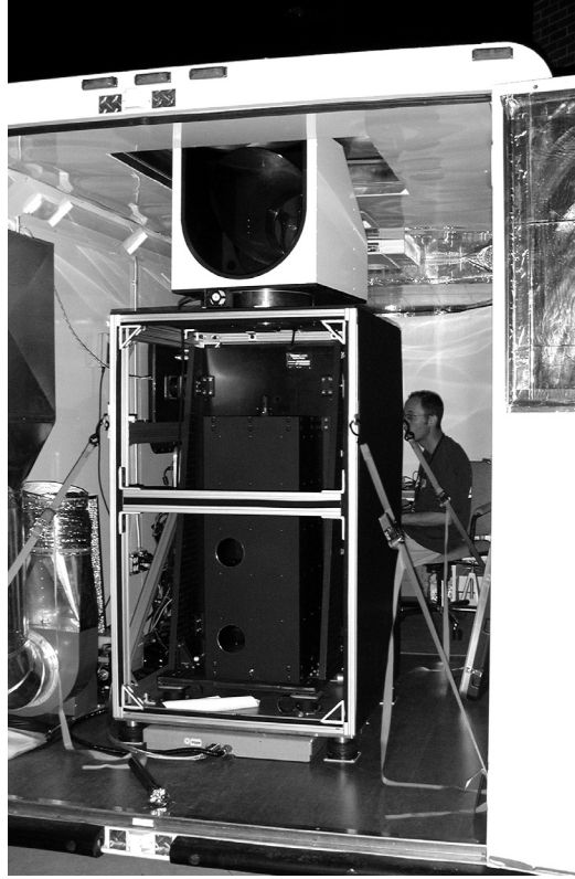
Figure 2. AGLITE lidar mounted vertically, viewed through open back door of trailer
