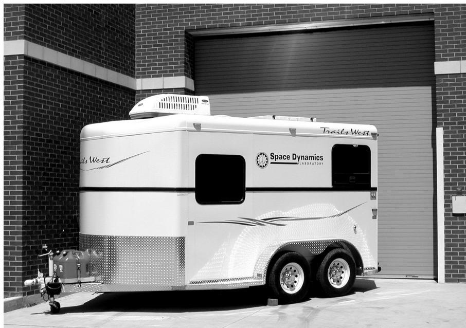
Figure 3. Field deployment trailer for AGLITE lidar
