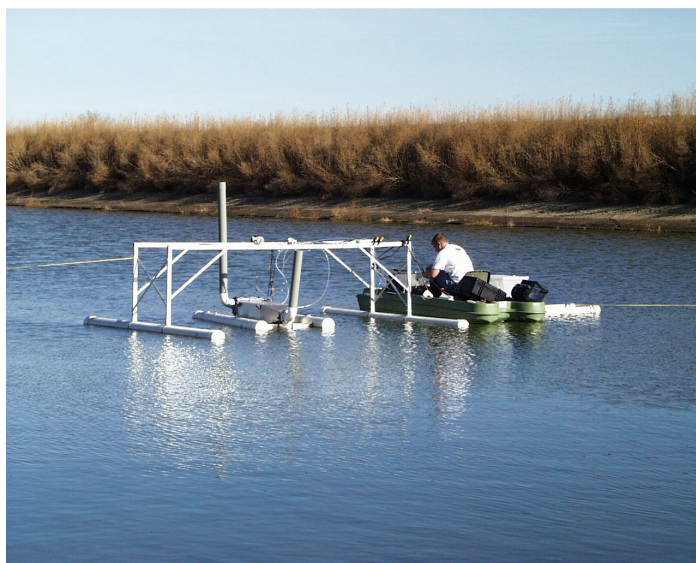
Figure 2. Collecting Emissions with a wind tunnel from a lagoon
