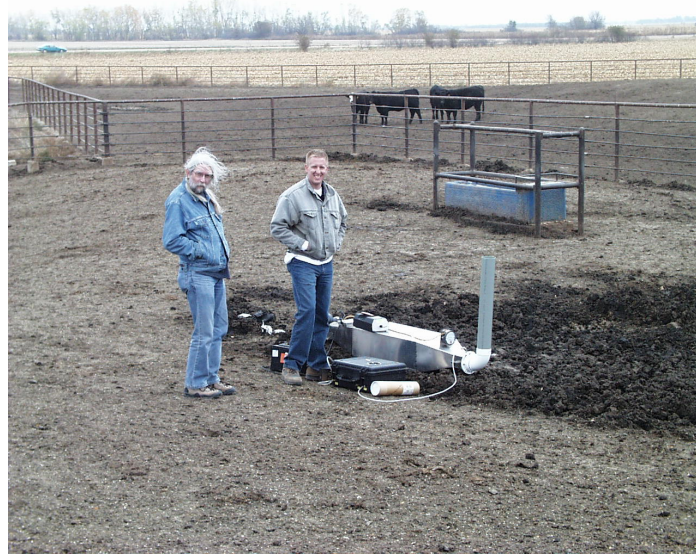
Figure 3. Collecting Emissions with a wind tunnel from a feedlot
