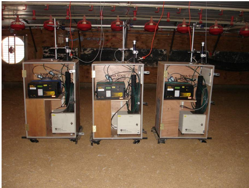
Figure 6. In-house particulate matter monitoring instruments for PM 10 , PM 2.5 , and TSP.
