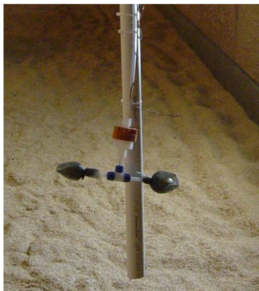
Figure 4. Gaseous emission in-house sample intake line with filters.
