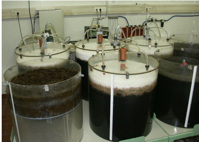
Figure 4. Measurement of gaseous emissions from manure storage facilities with dynamic chambers on lab scale
