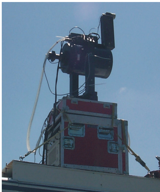
Figure 2. A photograph of the miniature elastic lidar set up to map particulates in the field. This instrument took the data in figures 3 and 4.
