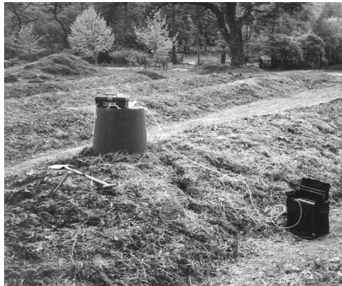
Figure 6. Measurement of linearity of concentration increase of a gas flux chamber on windrows of animal waste (straw bedding with cattle manure and pig manure) by a multigas monitor
