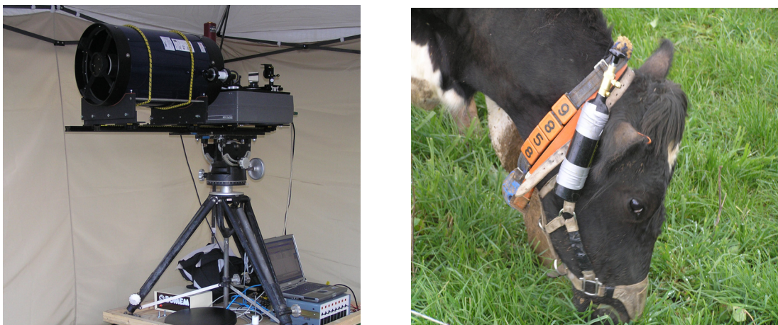
Figure 2. The open path FTIR spectrometer (left) and tracer release canister mounted on a grazing cow (right)
