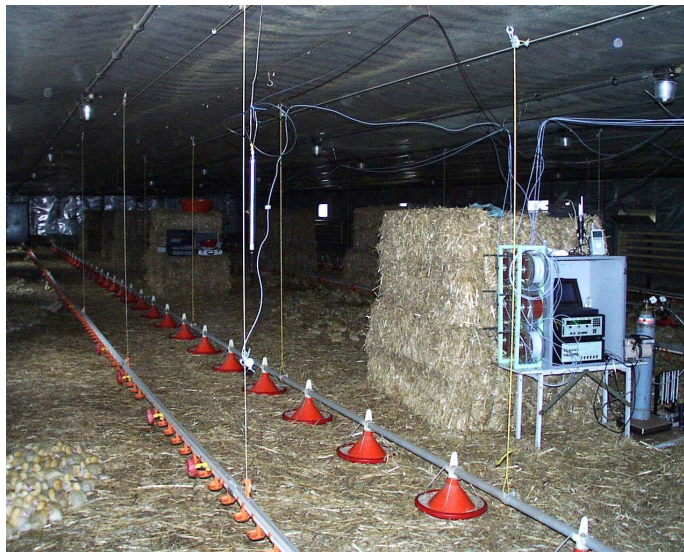
Figure 2. Equipment for gas analyses and gravimetric tracergas dosing in a forced ventilated poultry house
