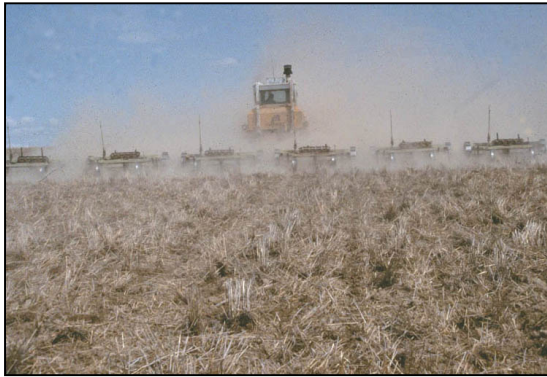
Figure 3. A rodweeder (2-cm square rotating rod) was operated 10 cm below the soil surface two to three times during late spring and summer to control weeds in summer fallow. Ample residue in the minimum tillage treatment (shown here) provides protection from wind erosion.
