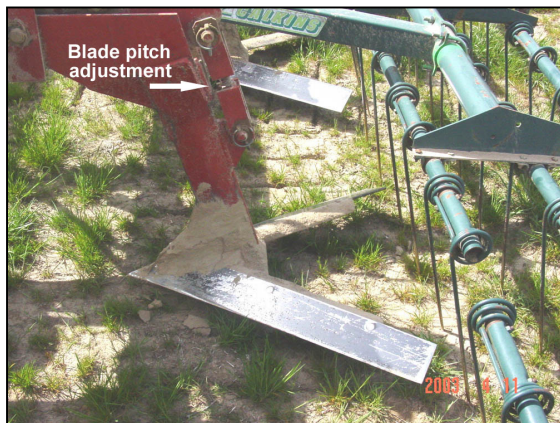
Figure 1. Haybuster™ undercutter V-sweep blade with attached 3-bar spring-tooth harrow. As a primary spring tillage implement, the undercutter completely severs capillary pores to halt liquid water movement toward the soil surface as required to retain seed-zone water in summer fallow.
