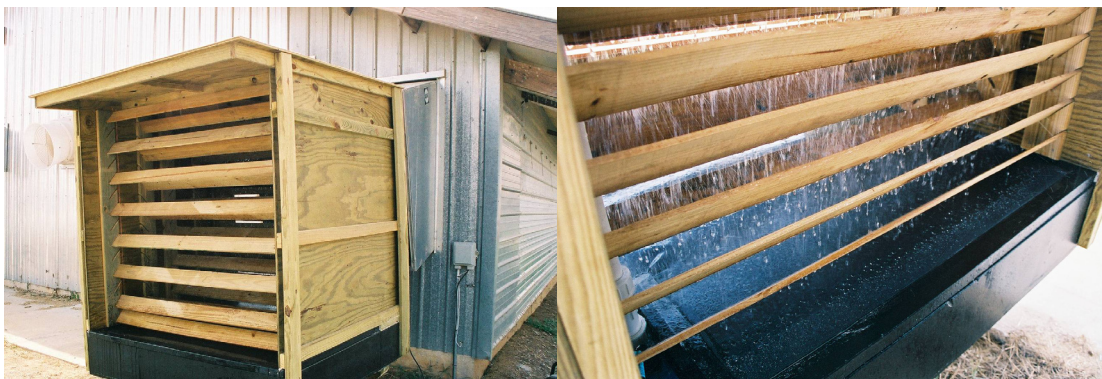
Figure 6. Ammonia and particulate scrubber for animal rearing facilities.
