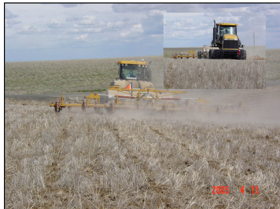
Figure 2. Primary spring tillage plus liquid aqua nitrogen injection with an undercutter V-sweep implement. Note that the majority of residue remains standing and undisturbed.
