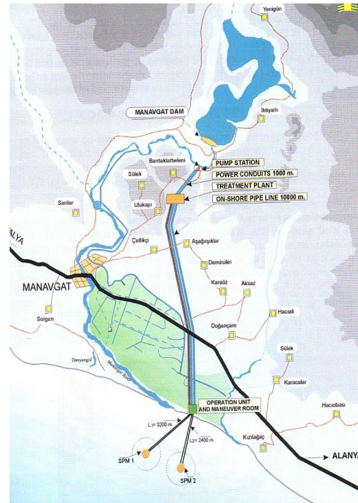
Figure 6: The Flow Chart and the plan view of the Manavgat project [15]
