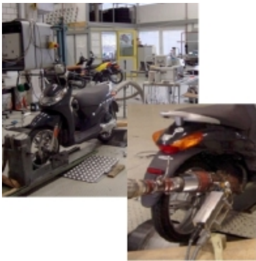
Fig. 1 : Investigated scooter Peugeot Looxor TSDI on the chassis dynamometer
