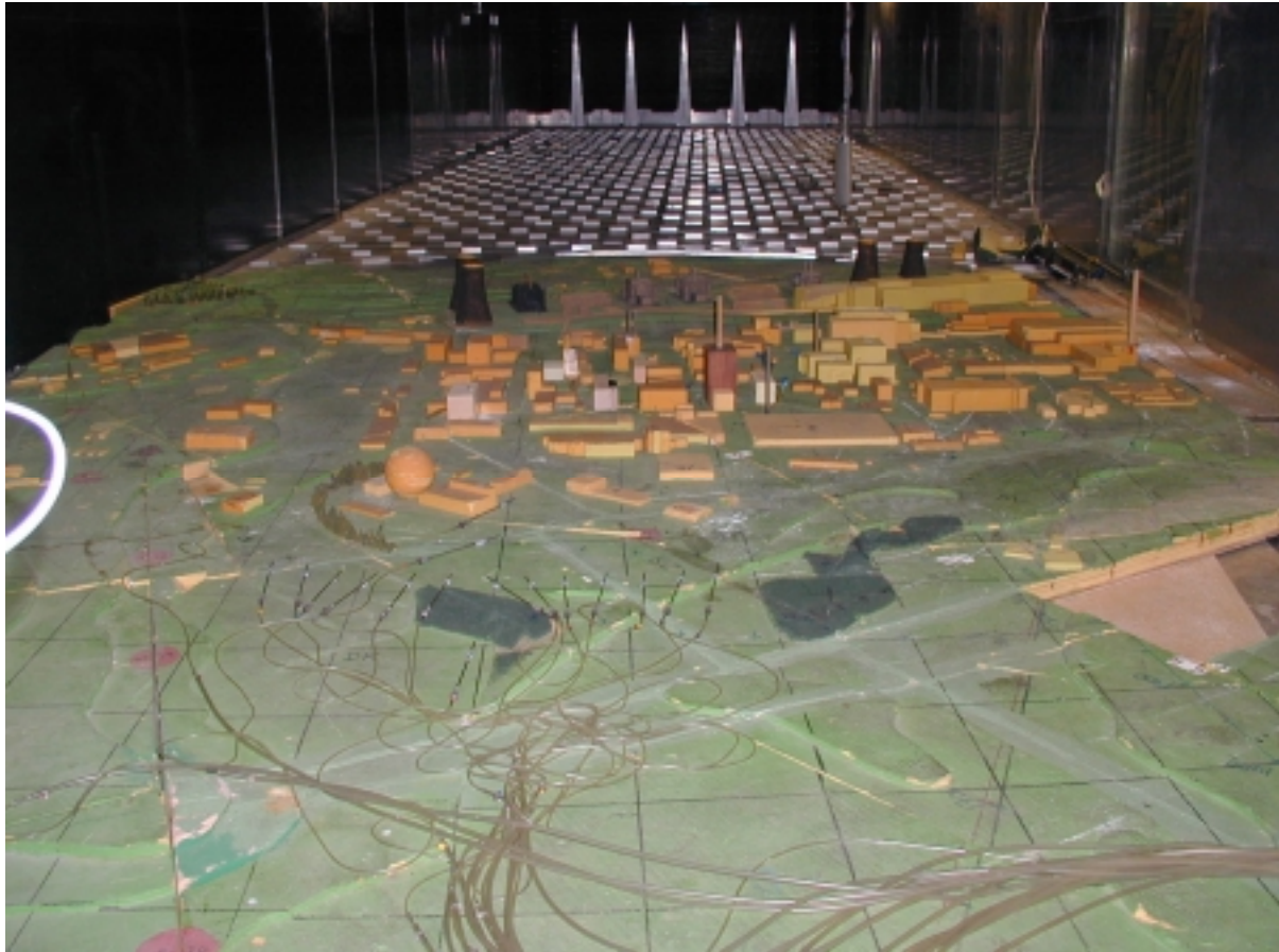
Figure 2: The 1:500 Sellafield wind tunnel model within the wind tunnel
