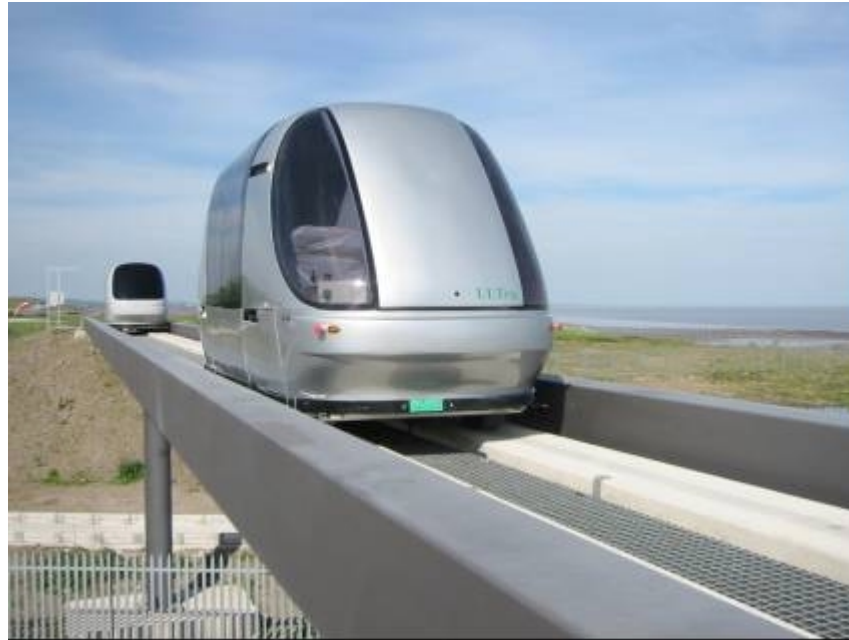
Figure 1 ULTra Vehicles on the Cardiff test track
