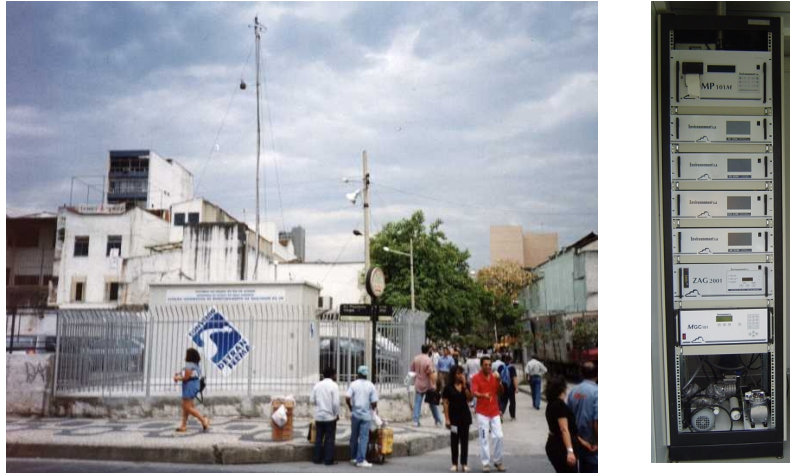
Figure 1 : Fixed station and analysers housed in 19'' rack cabinet
