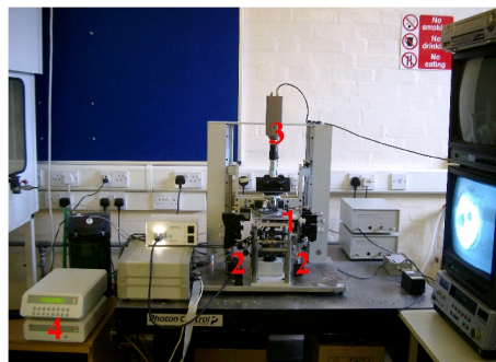
Fig. 2. Photography of the micromanipulation rig for measuring the adhesive force between particles. 1: hot stage; 2: micromanipulator; 3: microscope with CCD; 4: temperature controller.
