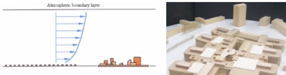
Figure 5: Atmospheric boundary layer and scale-model of the hospital
