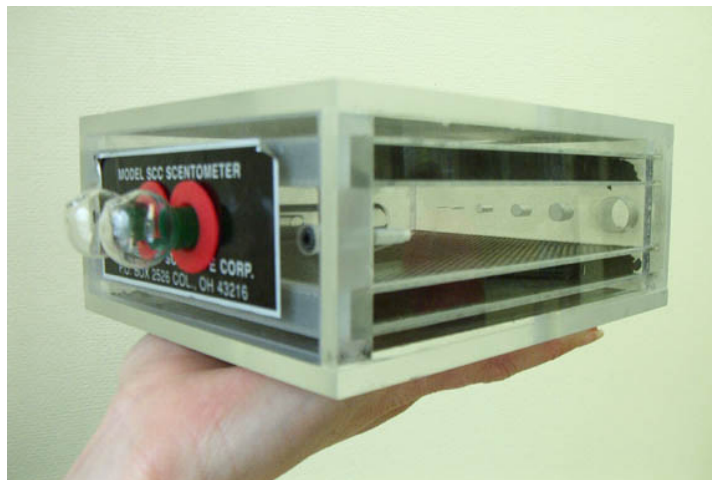
Figure 5. The Scentometer Field Olfactometer (Barnebey Sutcliffe Corp.). Note the two glass nostril ports to the left and the series of orifice holes at the back of the unit to the right in this photo.
