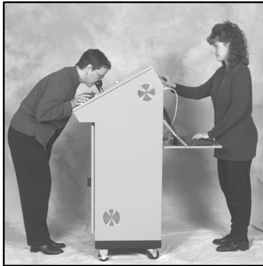
Figure 1. Assessor (left) sniffing at a dynamic dilution olfactometer. AC'SCENT Olfactometer photo courtesy of St. Croix Sensory, Inc.
