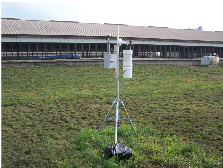
Figure 1. Particle and NH_3 samplers near pig barn
