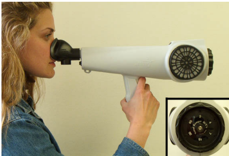
Figure 6. The Nasal Ranger® Field Olfactometer (St. Croix Sensory, Inc.). The inset picture shows a close-up of the orifice dial, which is located at the right side of the Nasal Ranger in this photo.
