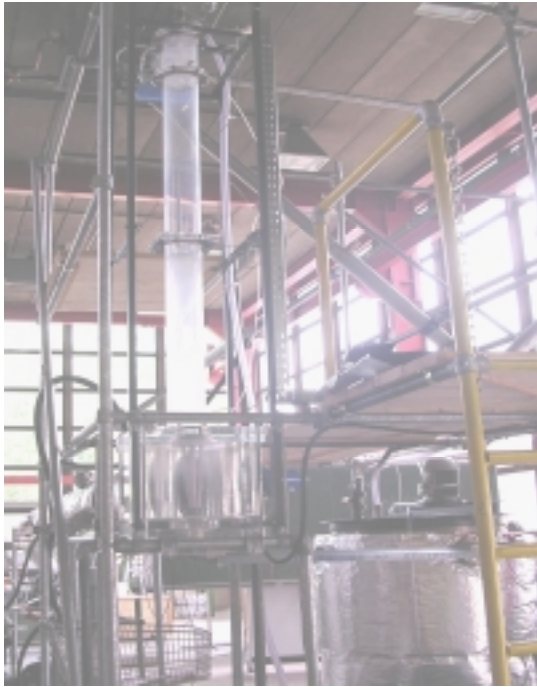
Figure 2. The \text{SO}_{2(g)} Scrubber Pilot Scale
